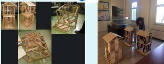
Wooden building models with removable laths and roof : which building combination behaves better /worse during the shaking.
